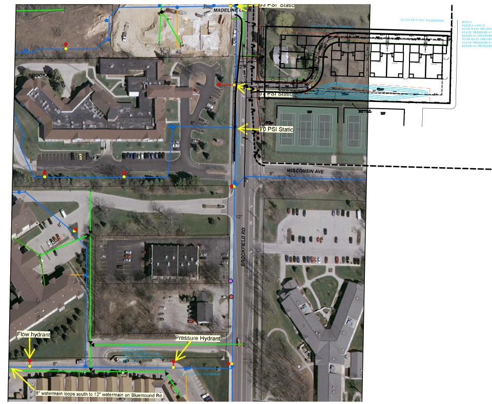
HYD #1 NOZZLE = 895.25 FLOW RATE 500 GPM STATIC PRESSURE = 54.7 PSI RESIDUAL PRESSURE = 52.8 PSI FLOW RATE 1000 GPM STATIC PRESSURE = 54.7 PSI RESIDUAL PRESSURE = 47.8 PSI
